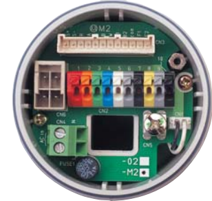
Color Coded Wiring Terminals
